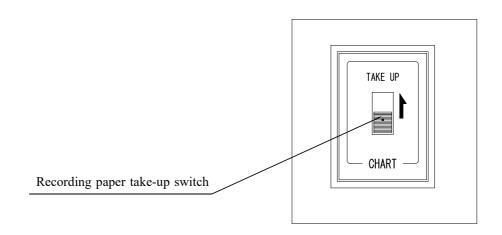
When this switch is set to "TAKE UP" side, the motor of the recording paper take-up device rotates and the recording paper can be taken up.
